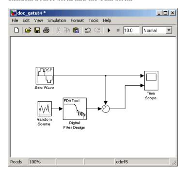
**3** Run your model and view the results in the **Time Scope** window. This window shows the original input signal and the signal with low frequency noise added to it.
