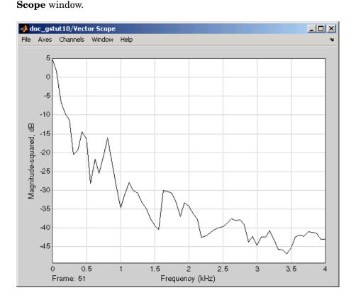
During the simulation, the **Vector Scope** window displays a series of frames output from the Periodogram block. Each of these frames corresponds to a window of the original speech signal. The data in each frame represents the power spectrum, or contribution of every frequency to the power of the original speech signal, for a given window.
